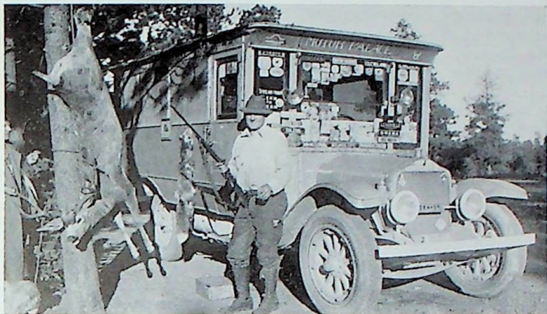
M. W. Trester's famous "Motor Palace" in which he and Mrs. Trester traveled from coast to coast and border to border. This wonder car was a large sky blue vehicle built on a Model 15-45 White, 4-ton truck Chassis. Cost, $16,000!
